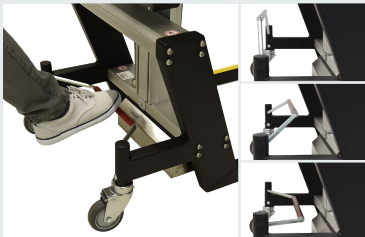
Figure 3: Brake Lever Position (Top to Bottom: Directional Lock, Free Wheeling, Set Brake)
