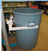
Barrel handle is secured on lifter arm.
